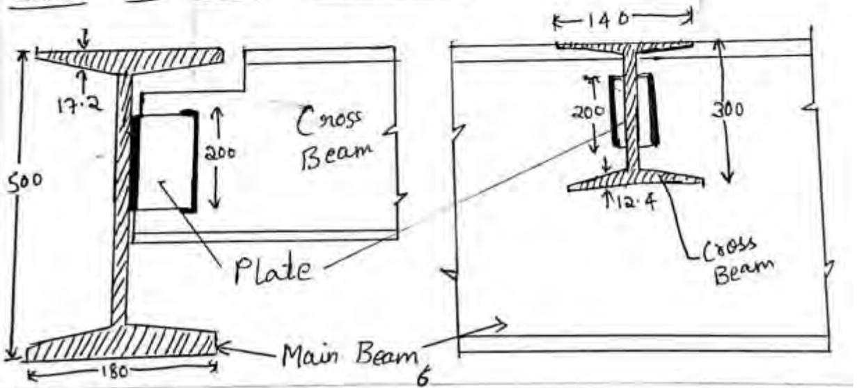
**Beam-column stiffened seat connection:**
