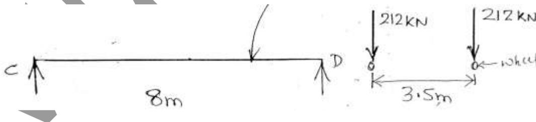
“The arrangement of wheel load for maximum BM is, the mid span is equi-distance from resultant of two wheel loads and any one load”.
