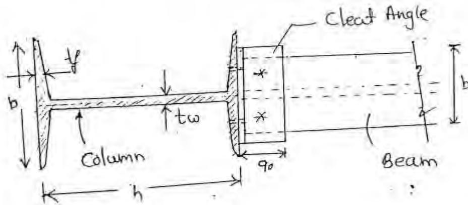
**Beam to column stiffened seat connection**
