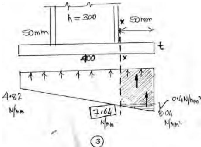
(C) Connection: Upward reaction on shaded area
