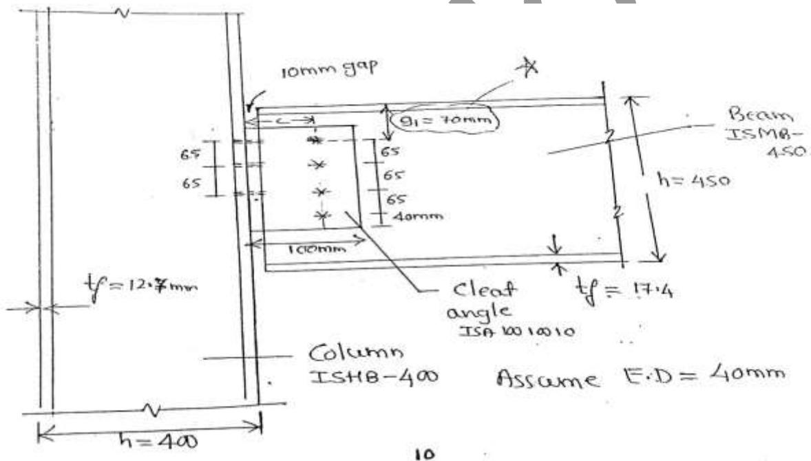
**Beam to column un-stiffened seat connection**
