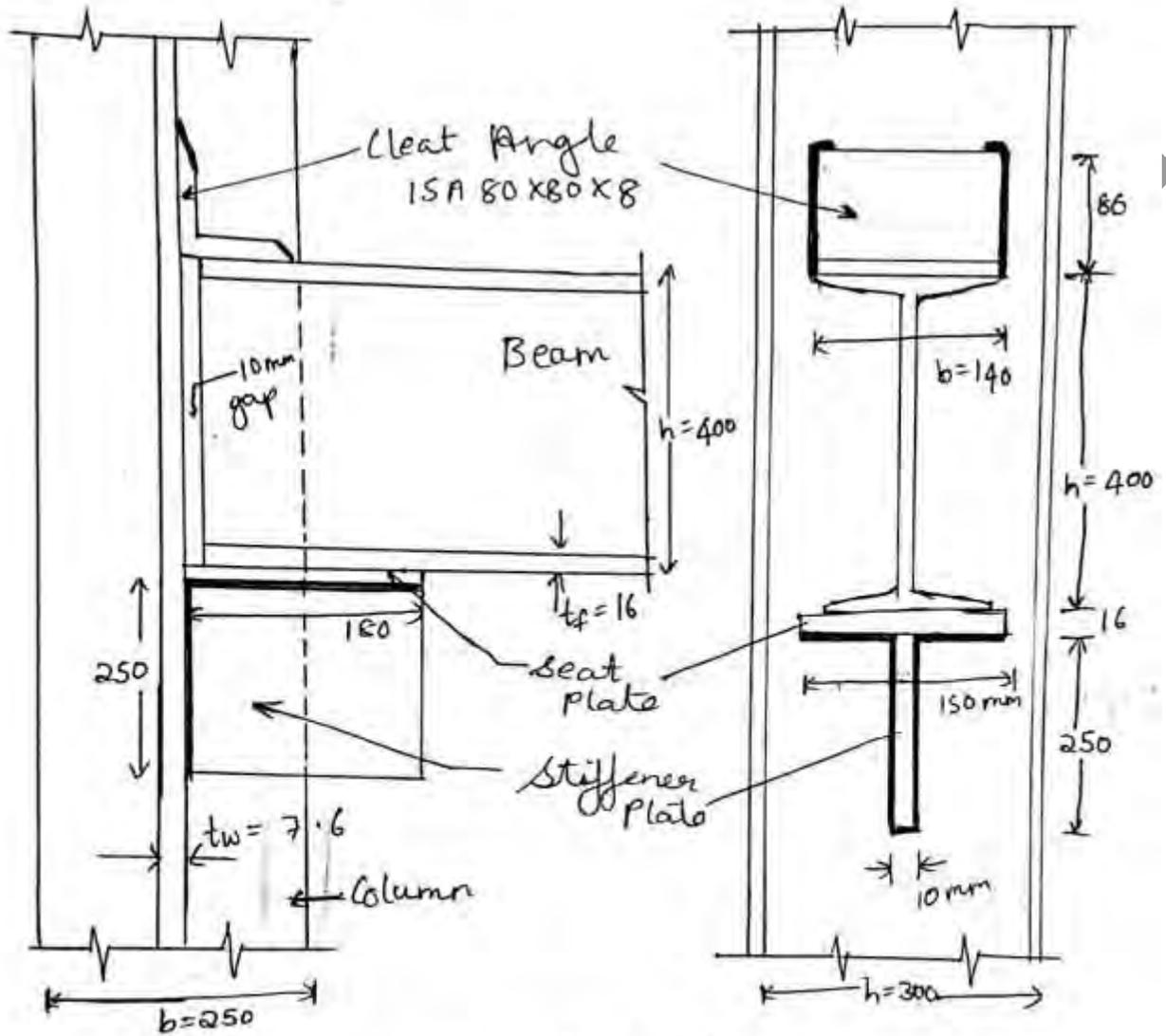
Beam is connected to the web
