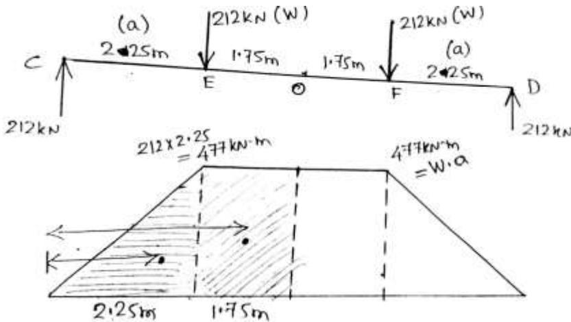
$$d)_{\text{load}} + d)_{\text{self wt}} = 10.67 \text{ mm}, E = 2 \times 10^5 \text{ N/mm}^2$$
