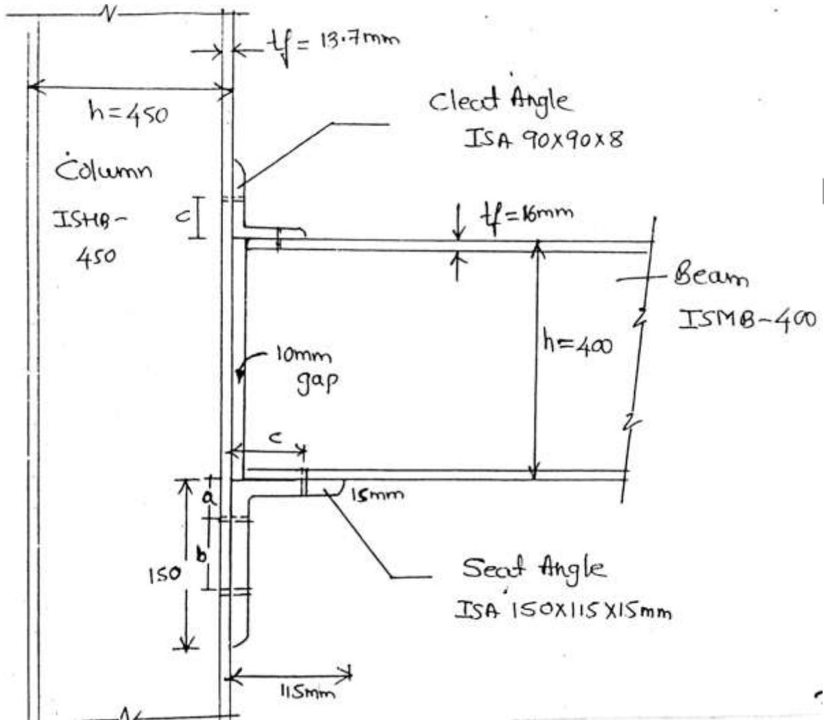
ISMB 400 @ 872 N/m by using a unstiffened seat connection.
