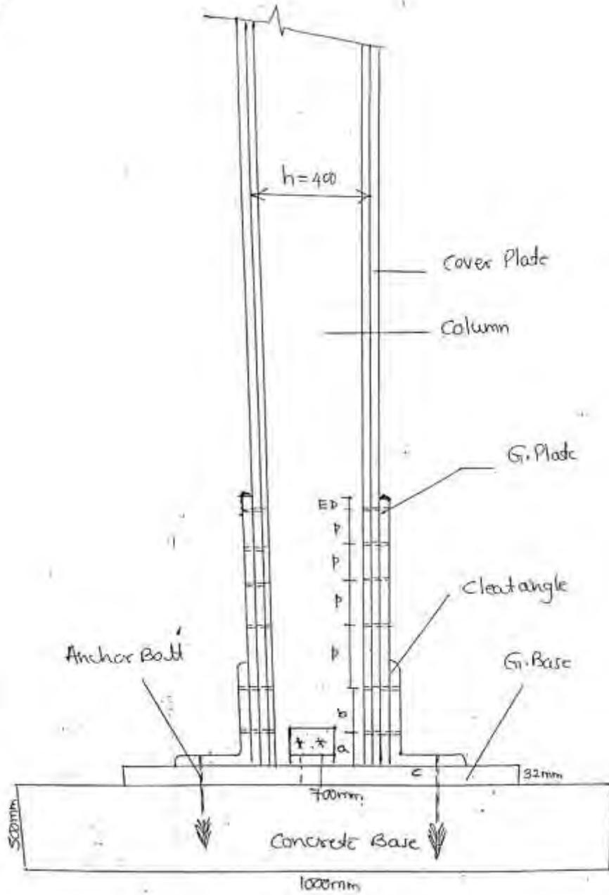
The column is connected to battens using welded connection size of the battens = 250mm\* 10mm spacing @ 700mm c/c.
