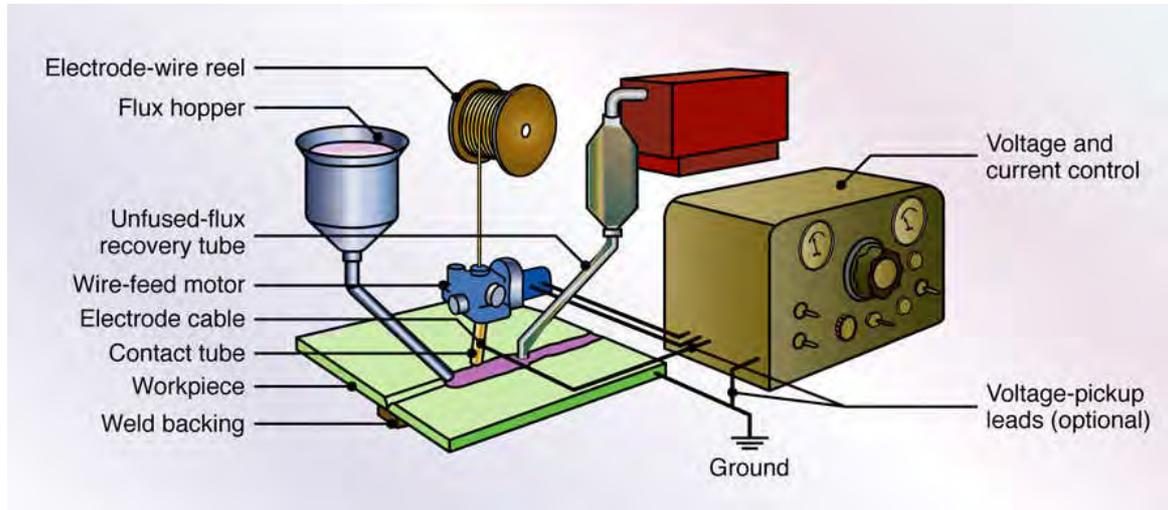
Figure 6: Schematic illustration of submerged-arc-welding (Source: Manufacturing Engineering and Technology, Fifth Edition, by Serope Kalpakjian and Steven Schmid. ISBN 0-13-148965-8. 2006 Pearson Education, Inc. PP 950)
