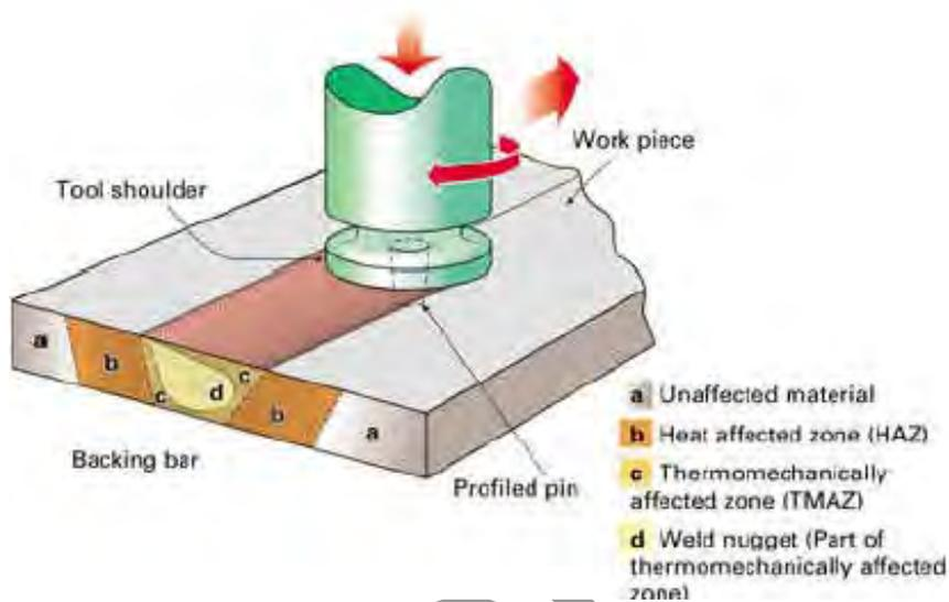
Figure 8: Schematic diagram of FSW (Nicholas et al 2002)
