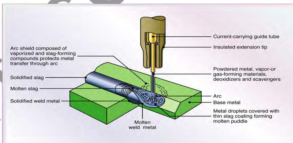
Figure 5: Schematic illustration of the flux-cored arc-welding process
