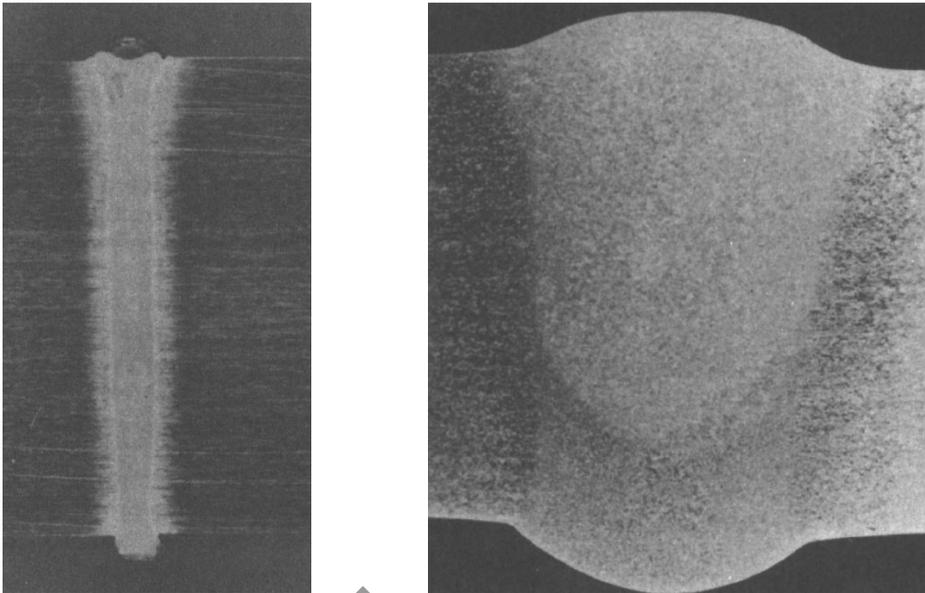
Figure 10: Comparison of the size of weld beads: (a) Laser beam or electron beam welding (b) Tungsten arc welding (Source: Manufacturing Engineering and Technology, Fifth Edition, by Serope Kalpakjian and Steven Schmid. ISBN 0-13-148965-8. 2006 Pearson Education, Inc. PP 957)
