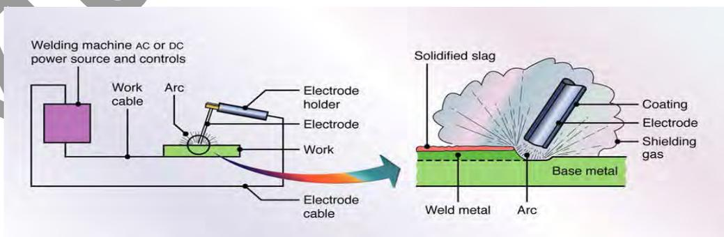
Figure 3: Schematic illustration of shielded metal arc welding
