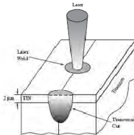
Figure 11: Schematic illustration of laser welding (Sergio and Lima 2005)
