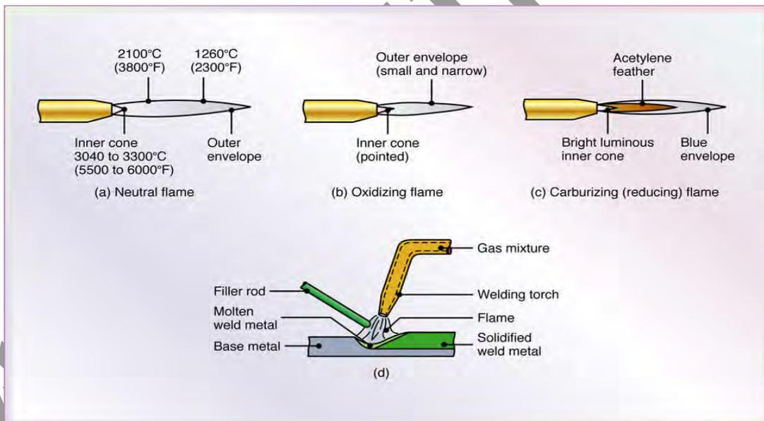
Figure 2: Schematic illustration of three basic oxyacetylene flames (a-c), (d) The principle of oxyfuel-gas welding operation (Source: Manufacturing Engineering and Technology, Fifth Edition, by Serope Kalpakjian and Steven Schmid. ISBN 0-13-148965-8. 2006 Pearson Education, Inc. PP 942
