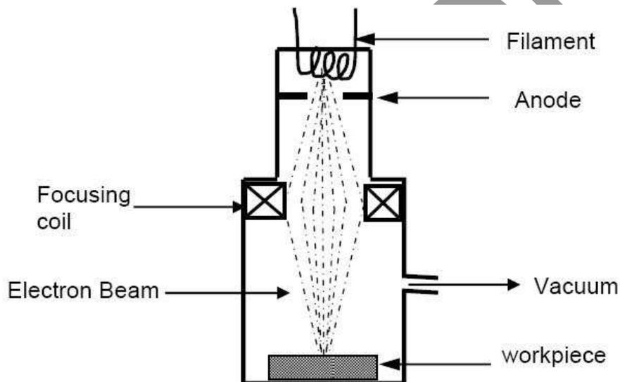
Figure 9: Schematic illustration of Electron Beam Welding (EBW) (Source: MAS 2007)
